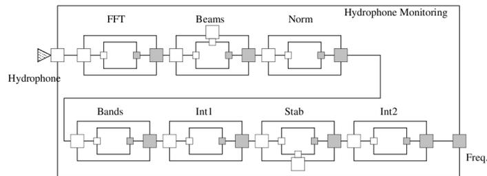
**Fig. 2:** Array-OL specification of a hydrophone monitoring application.
