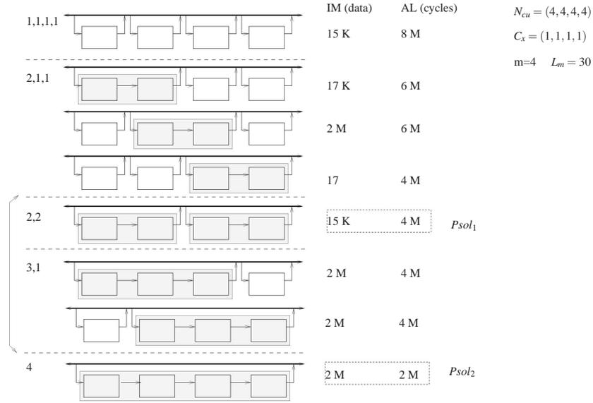
**Fig. 1:** Example of an exploration for a 4-tasks application. Dependencies impose to the solutions merging the 2 central tasks to use the largest internal memories.
